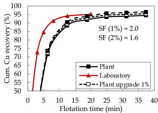
Fig. 9. Rougher vs. batch response for increases in industrial recovery (upgrade)
