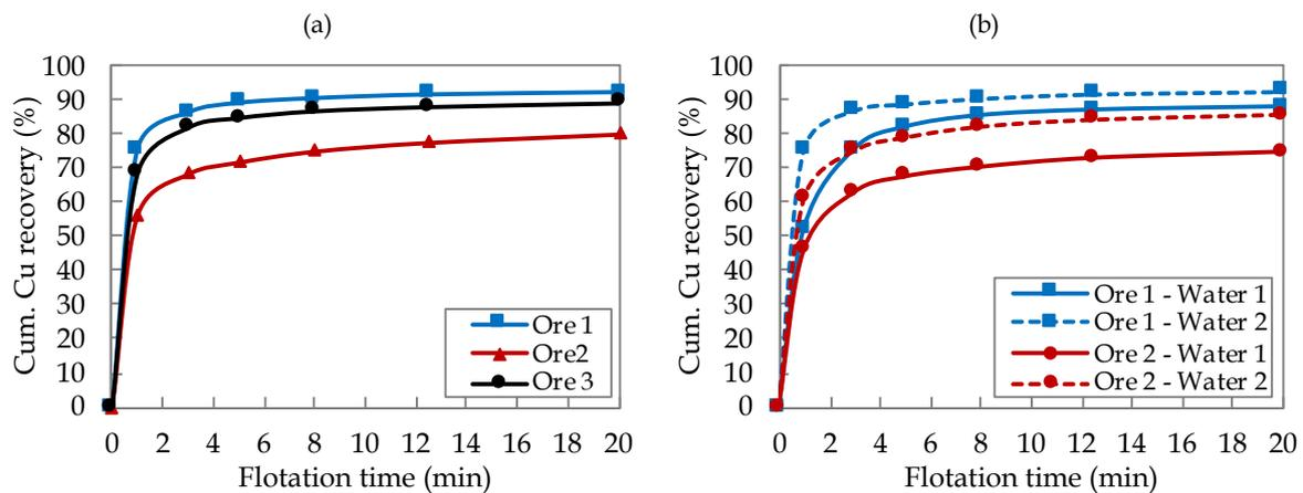
Fig. 6. Batch responses for case A, when changing: (a) ore type, and (b) water quality
