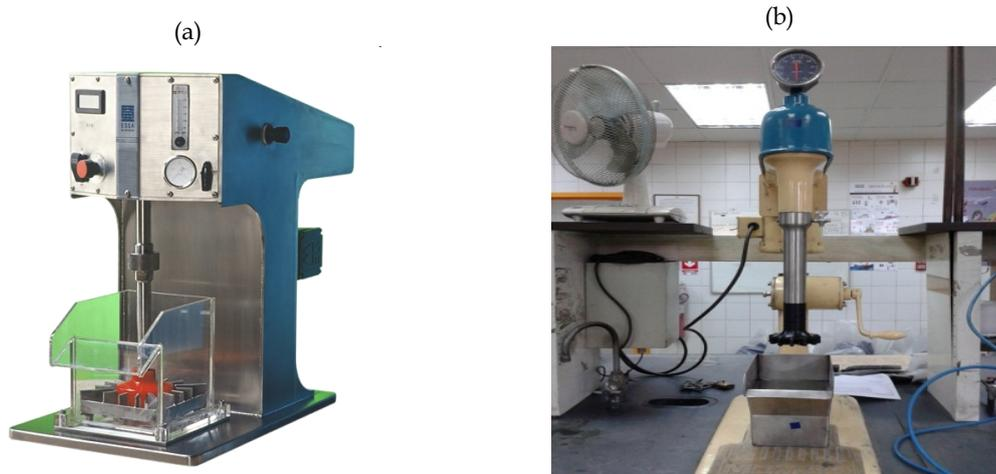
Fig. 1. Examples of batch flotation cells: (a) Agitair and (b) Denver
