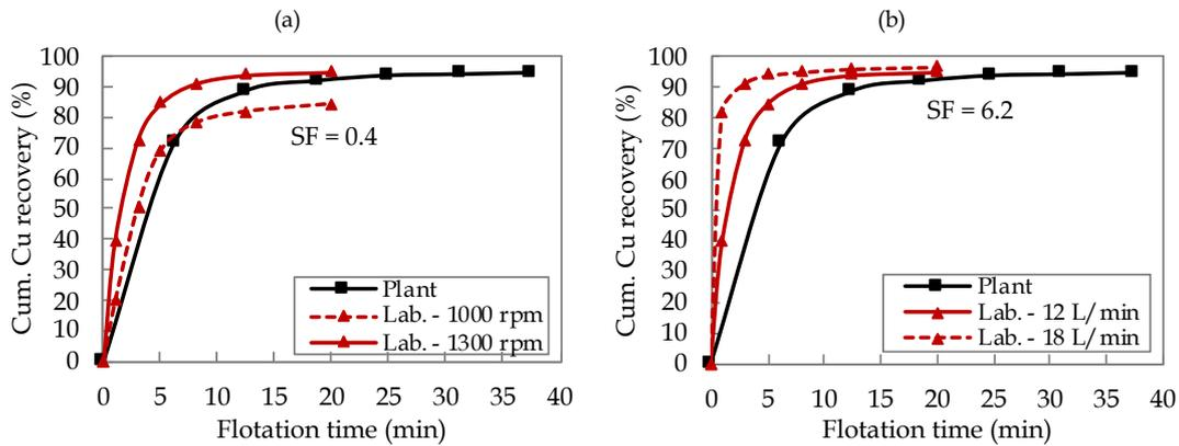
Fig. 8. Rougher vs. batch response for changes in (a) impeller speed, and (b) gas flowrate
