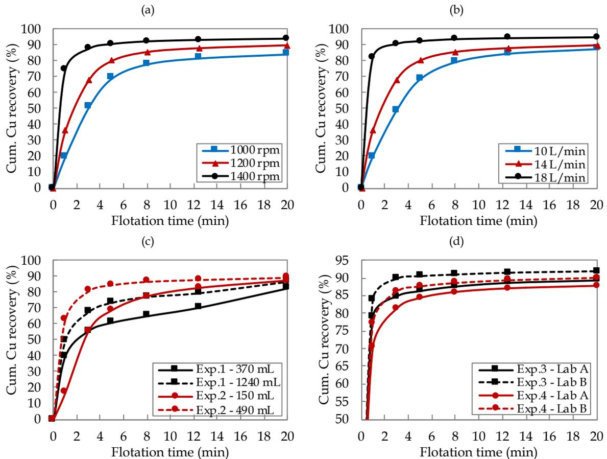
Fig. 3. Batch responses for case A, when changing: (a) impeller speed, (b) gas flowrate, (c) volume of makeup water, and (d) laboratory
