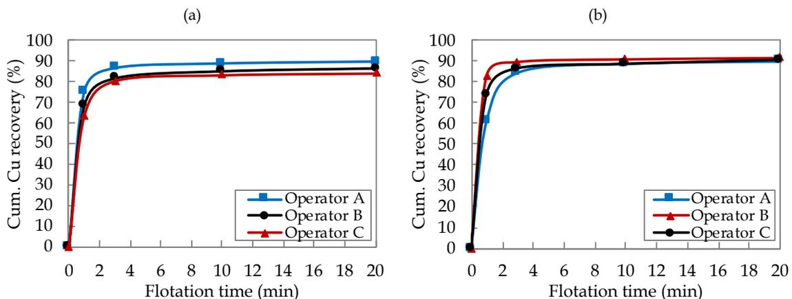
Fig. 5. Batch responses for case B, when changing the operator, using (a) primary and (b) secondary ore
